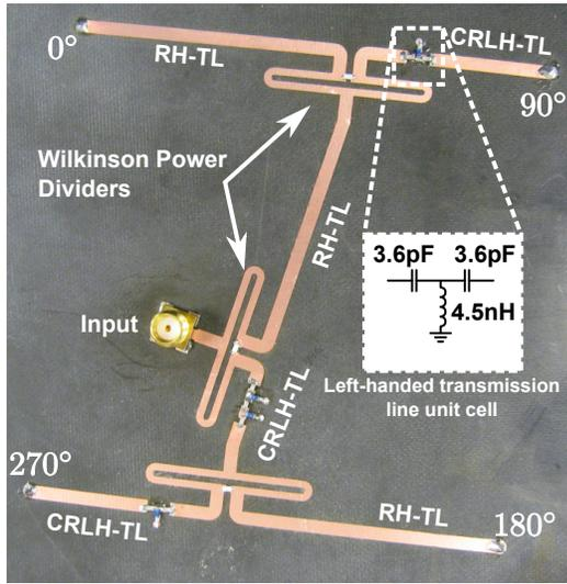
Fig. 2. Prototyped CRLH feed network used to achieve wideband CP radiation. The first power dividing/CRLH stage provides  $180^\circ$  phase delay between the two branches, and each subsequent stage provides  $90^\circ$  phase.
