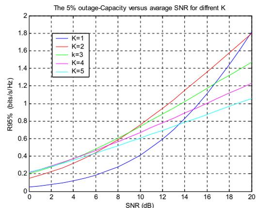
Capacity with  $q=5\%$  outage probability versus SNR for pulsed-OFDM systems with different upsampling rates
