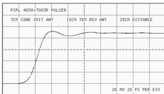
Transmission ( $l = 25\text{cm}$ ) between 7cm cone and 15cm TEM horn\*
