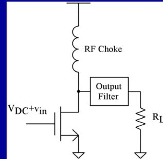
$$P_{dc}(\text{dBm}) = P_{total} + \text{Backoff} + 10\log\left(\frac{1}{\text{Eff}}\right)$$
