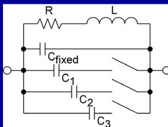
$$\left| \frac{Z_{\max}}{Z_{\min}} \right| = \left( \frac{\omega_{0,\max}}{\omega_{0,\min}} \right)^2$$
