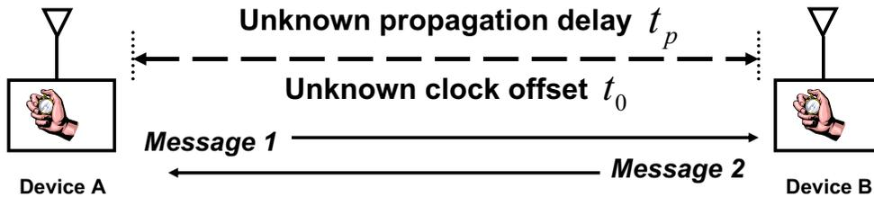
$$T_{2AR} = T_{2BT} - t_o + t_p$$
