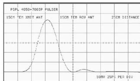
Transmission ( $l = 25\text{cm}$ ) between identical 15cm long TEM horns\*
