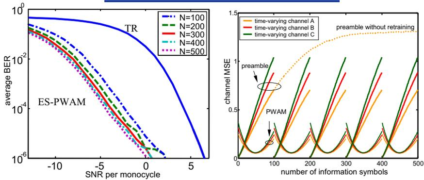
At high SNR: 250Kbps (TR) 495Kbps (N=100) 499Kbps (N=500)
