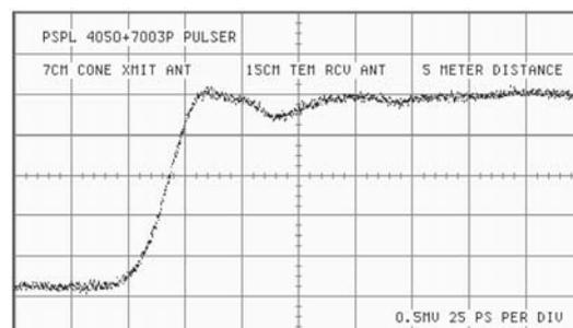
Transmission ( $l = 5\text{m}$ ) between 7cm cone and 15cm TEM horn\*
