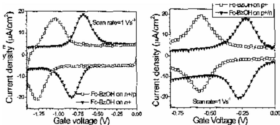
Figure 7a CyV of Fc-BzOH on n+ and n+/p diode: effect of forward-biased diode characteristics on redox peak potentials. Doping density of the n+ region is in the order of  $1 \times 10^{21} \text{ cm}^{-3}$ .
