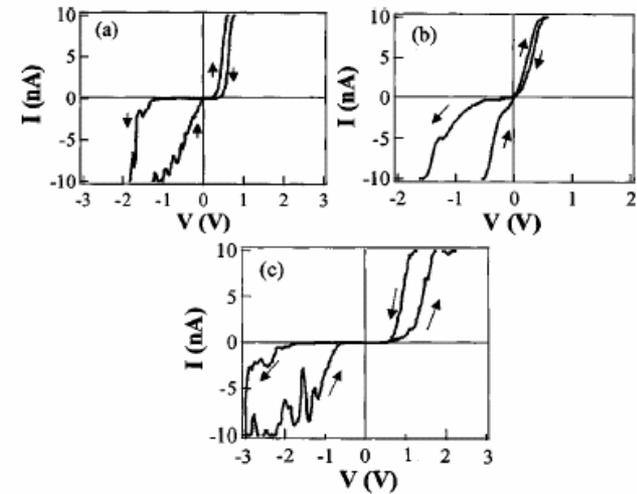
FIG. 3. Typical  $I-V$  curves of molecular devices. (a), (b), and (c) correspond to molecules **a**, **b**, and **c** shown in Fig. 2, respectively.
