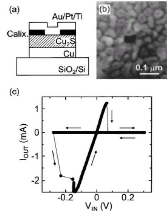
FIG. 1. (a) Schematic view of nanometer-scale switch using a  $\text{Cu}_2\text{S}$  film sandwiched between Cu film and a top electrode (Au/Pt/Ti). (b) Plane view of top electrode with a hole in the center. (c) Current–voltage characteristics of the device with a  $0.03 \mu\text{m}$  hole.
