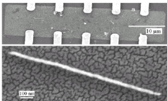
**Figure 1.** SEM image of the NanoCell after assembly of the Au nanowires and **1**. The top image shows the five juxtaposed pairs of fabricated leads across the NanoCell, and some Au nanowires are barely visible on the internal rectangle of the discontinuous Au film. The lower image is a higher magnification of the NanoCell's central portion showing the disordered discontinuous Au film with an attached Au nanowire, which is affixed via the OPE-dithiol (not observable) derived from **1**.
