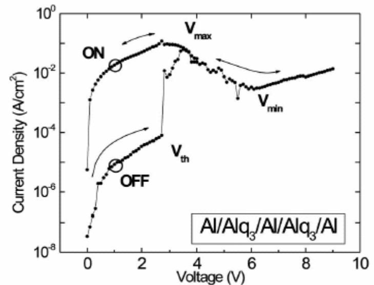
FIG. 3. Current-voltage characteristic of an Al (50 nm)/Alq<sub>3</sub> (50 nm)/Al (5 nm)/Alq<sub>3</sub> (50 nm)/Al (50 nm) device. The fundamental parameters of the bistable behavior are indicated. The ON and OFF states are set at voltages close to  $V_{\max}$  and  $V_{\min}$ , respectively, and read at 1 V. The transition from the OFF to the ON state occurs at the threshold voltage ( $V_{\text{th}}$ ).
