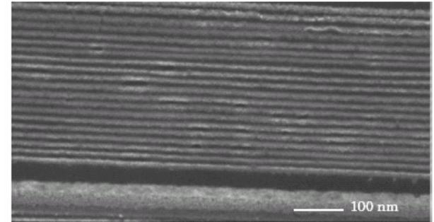
**Figure 2. Array of nanowires**, each approximately 5 nm in diameter. The lattice constant is 15 nm. Certain materials parameters important to solid-state devices, such as the average density of dopant atoms, no longer hold meaning at these nanoscale dimensions. At this size scale, however, chemical control over molecular properties is highly developed.
