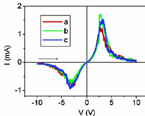
**Figure 2.**  $I(V)$  characteristics of the NanoCell at 297 K. Curves a, b, and c are the first, second, and third sweeps, respectively ( $\sim 40$  s/scan). The PVRs in curve c are 23:1 and 32:1 for the negative and positive switching peaks, respectively. The black arrow indicates the sweep direction of negative to positive.
